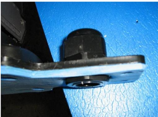
**Step 4.** Attach gland to base. Fully tighten bottom gland screw.
