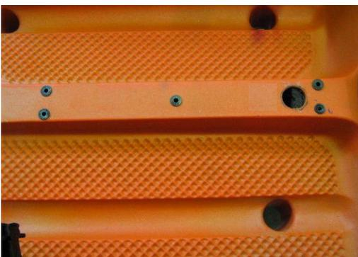
**Step 3.** Fit well-nuts into the 9mm holes.
